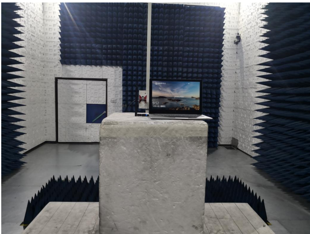
FCC RADIATED EMISSION TEST SETUP ABOVE 1GHZ
