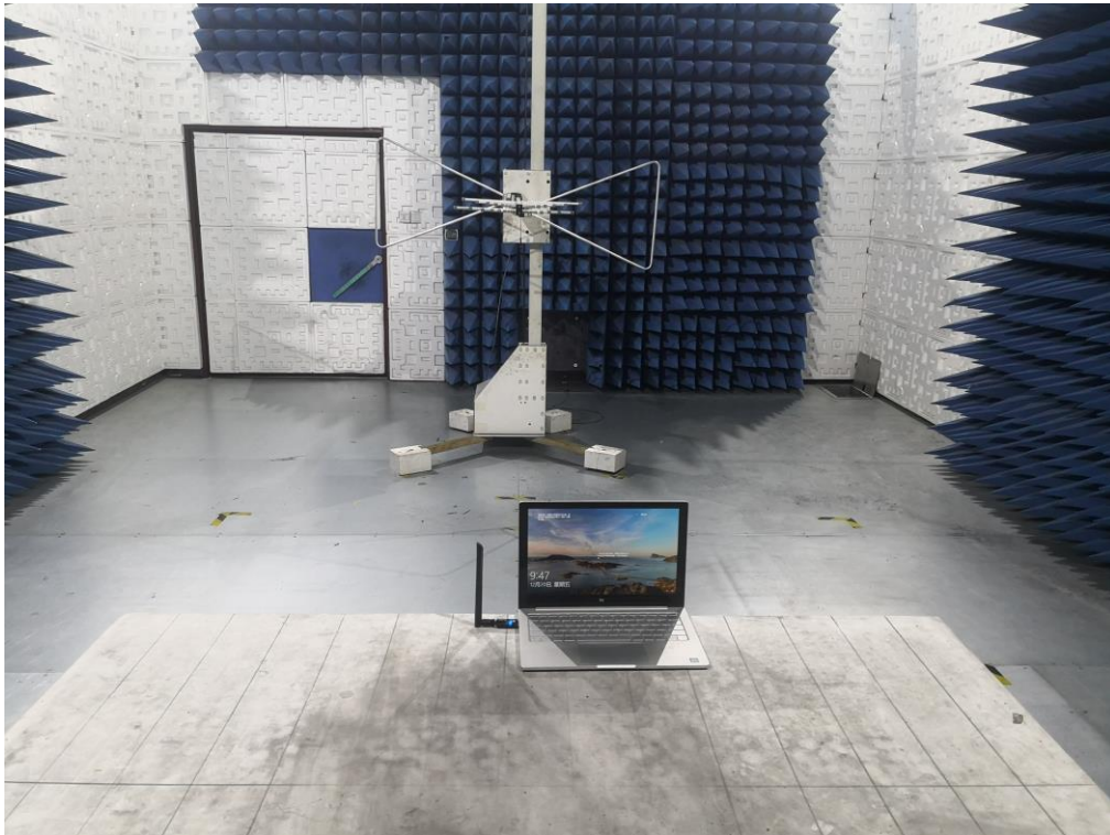
FCC RADIATED EMISSION TEST SETUP ABOVE 1GHZ
