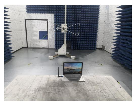
FCC RADIATED EMISSION TEST SETUP ABOVE 1GHZ
