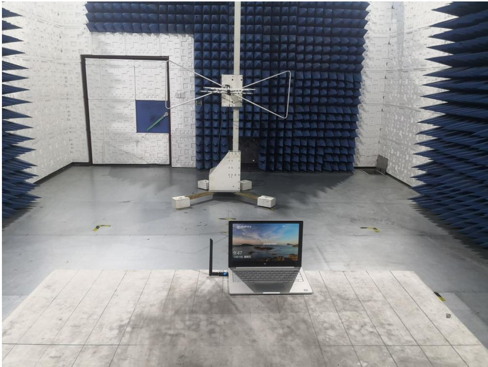
FCC RADIATED EMISSION TEST SETUP ABOVE 1GHZ
