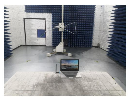
FCC RADIATED EMISSION TEST SETUP ABOVE 1GHZ
