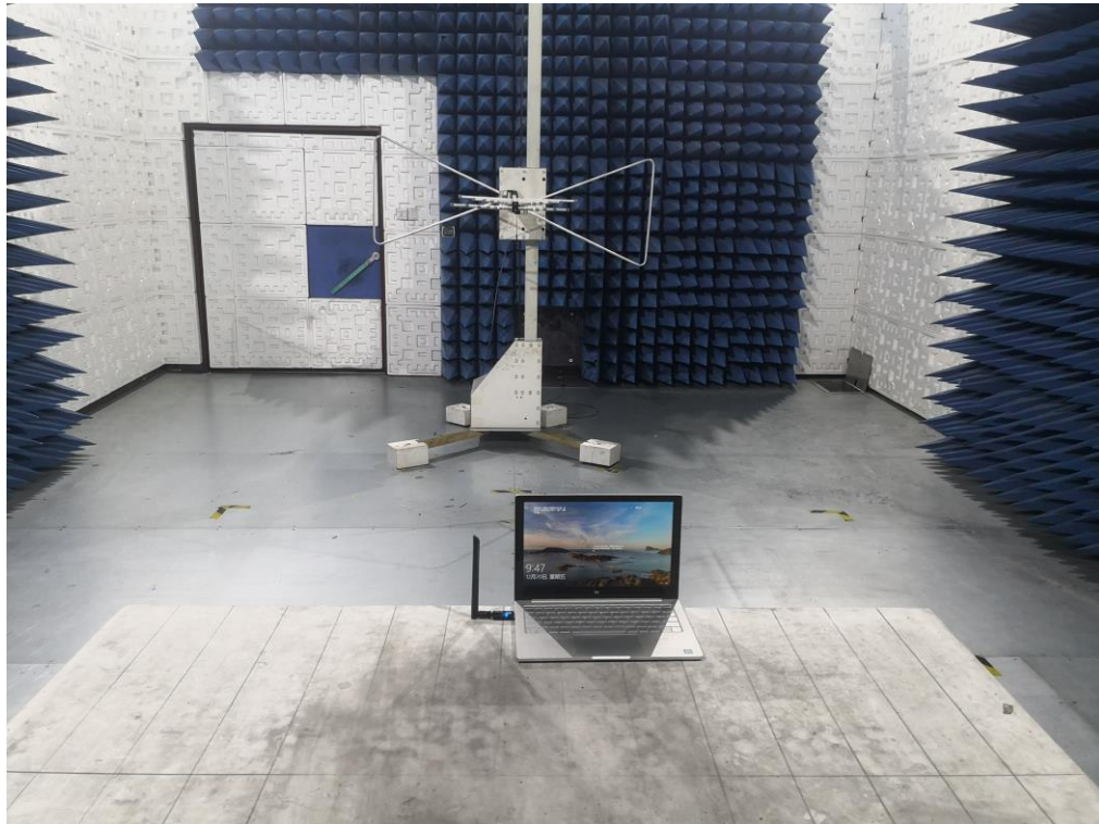
FCC RADIATED EMISSION TEST SETUP ABOVE 1GHZ
