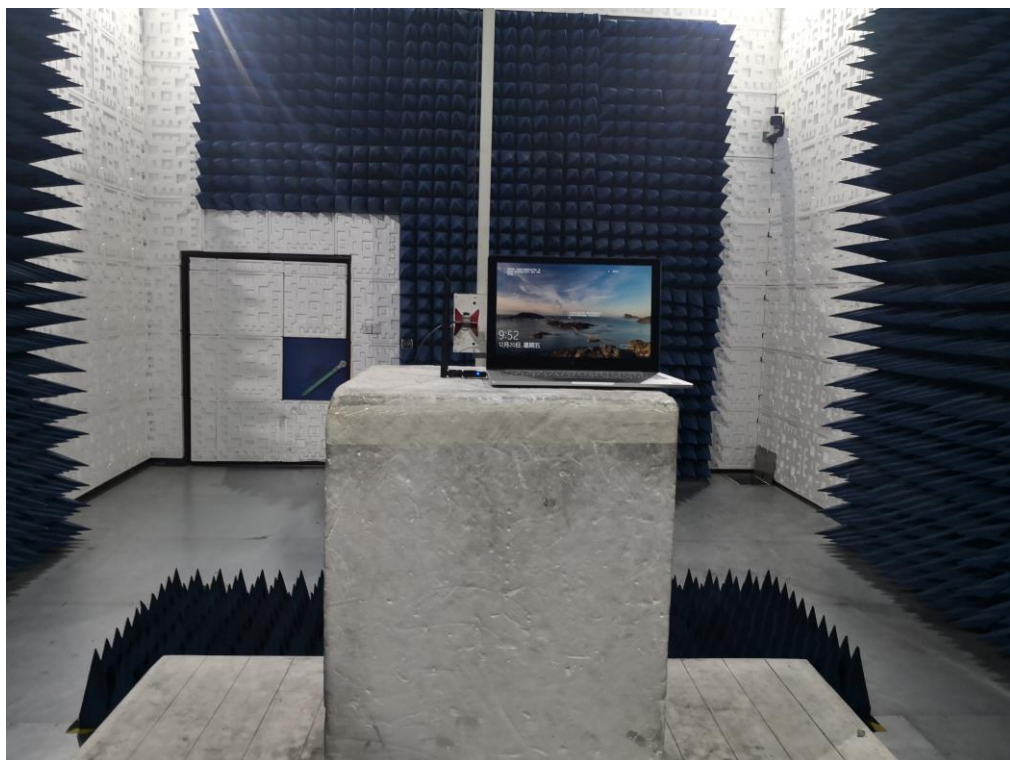
FCC RADIATED EMISSION TEST SETUP ABOVE 1GHZ
