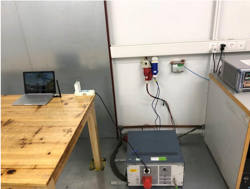
FCC RADIATED EMISSION TEST SETUP BELOW 1GHZ
