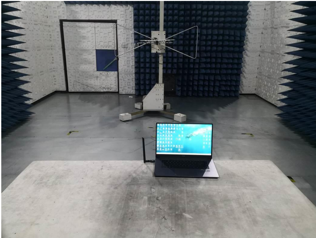
FCC RADIATED EMISSION TEST SETUP BELOW 1GHZ
