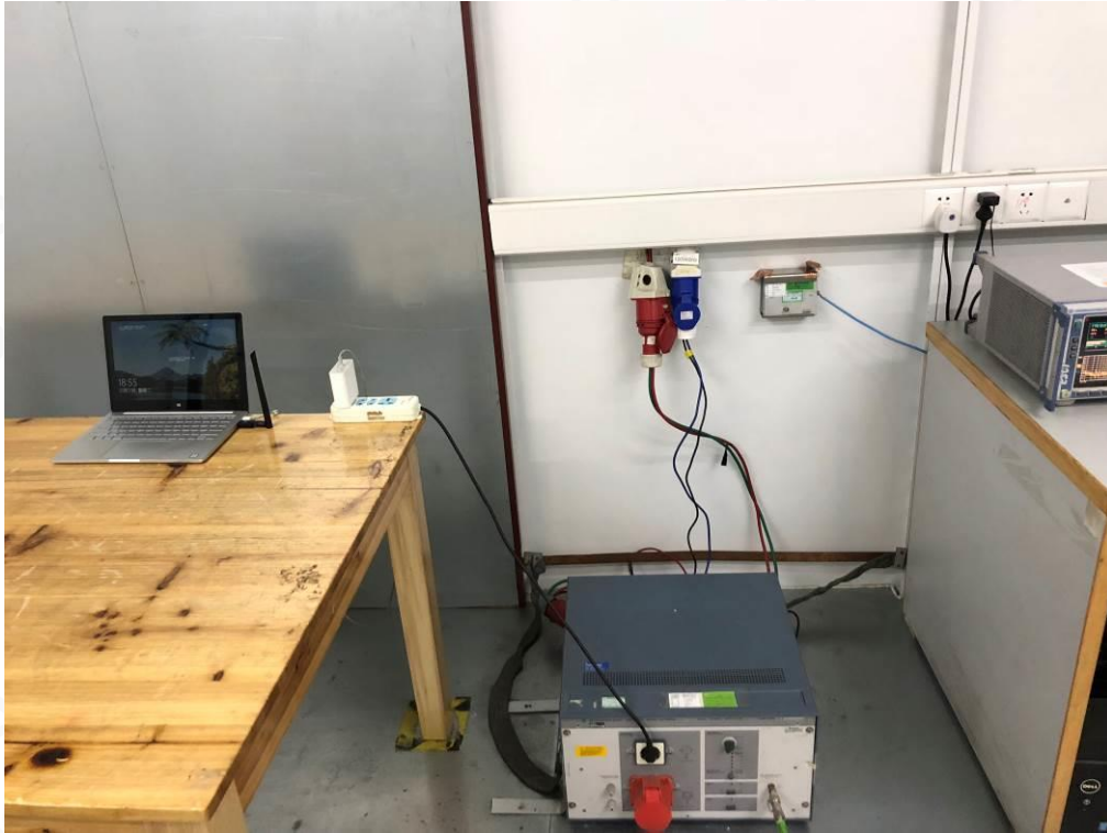
FCC RADIATED EMISSION TEST SETUP BELOW 1GHZ
