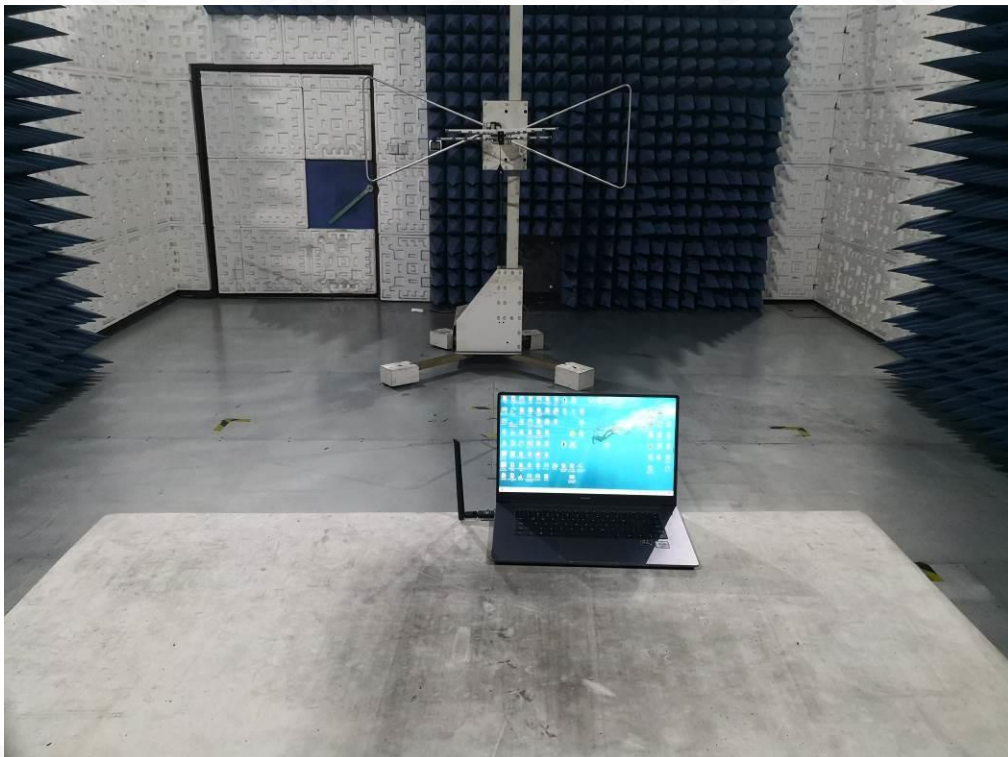
FCC RADIATED EMISSION TEST SETUP BELOW 1GHZ
