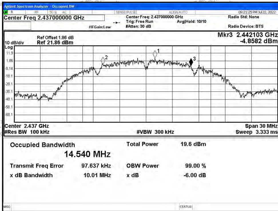
6dB Bandwidth NVNT b 2437MHz Ant1
