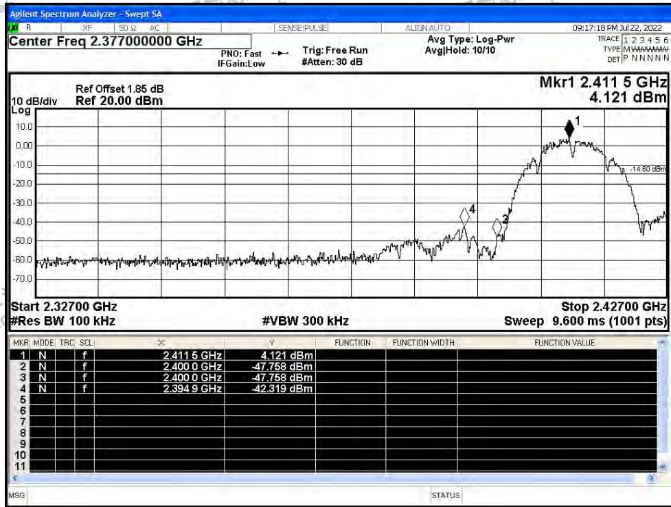
Band Edge NVNT b 2412MHz Ant1 Emission
