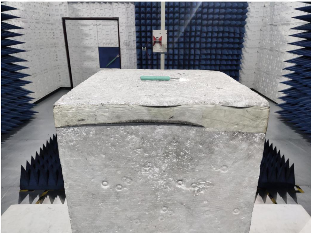
FCC RADIATED EMISSION TEST SETUP ABOVE 1GHZ
