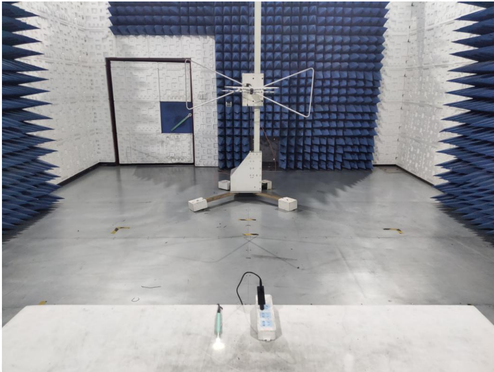
FCC RADIATED EMISSION TEST SETUP ABOVE 1GHZ
