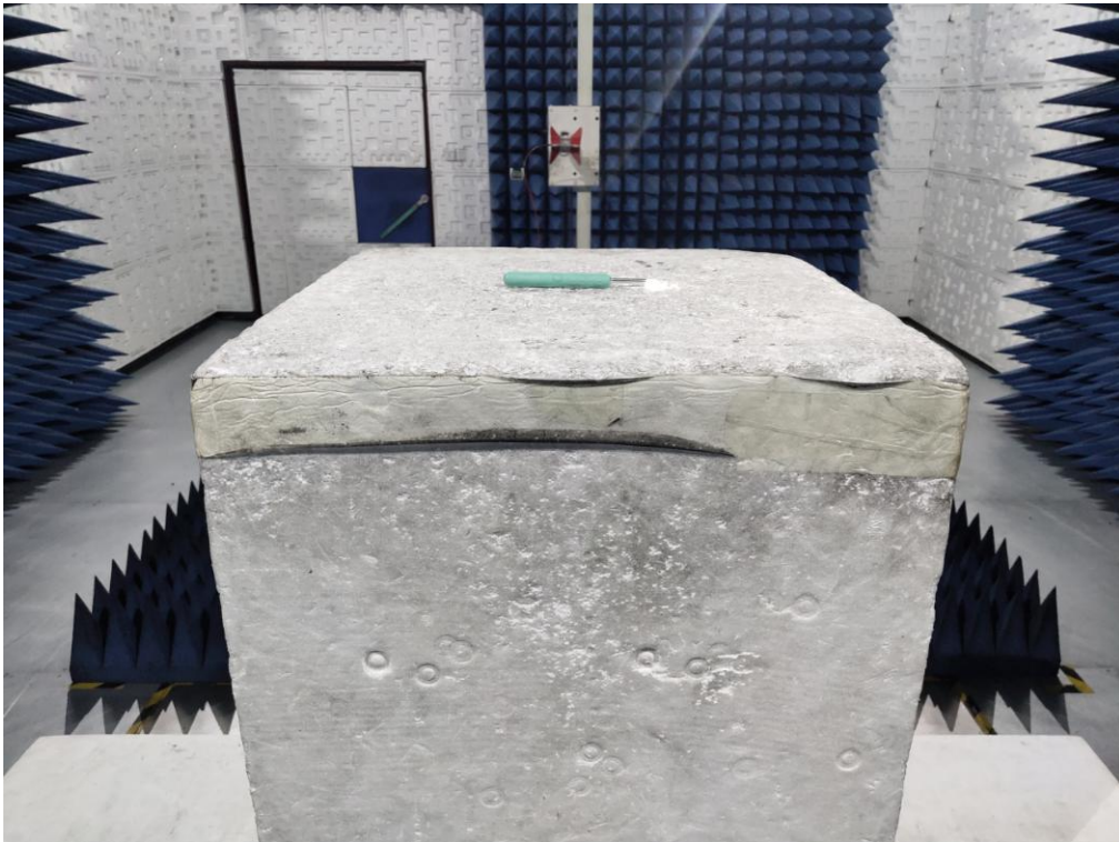
FCC RADIATED EMISSION TEST SETUP ABOVE 1GHZ
