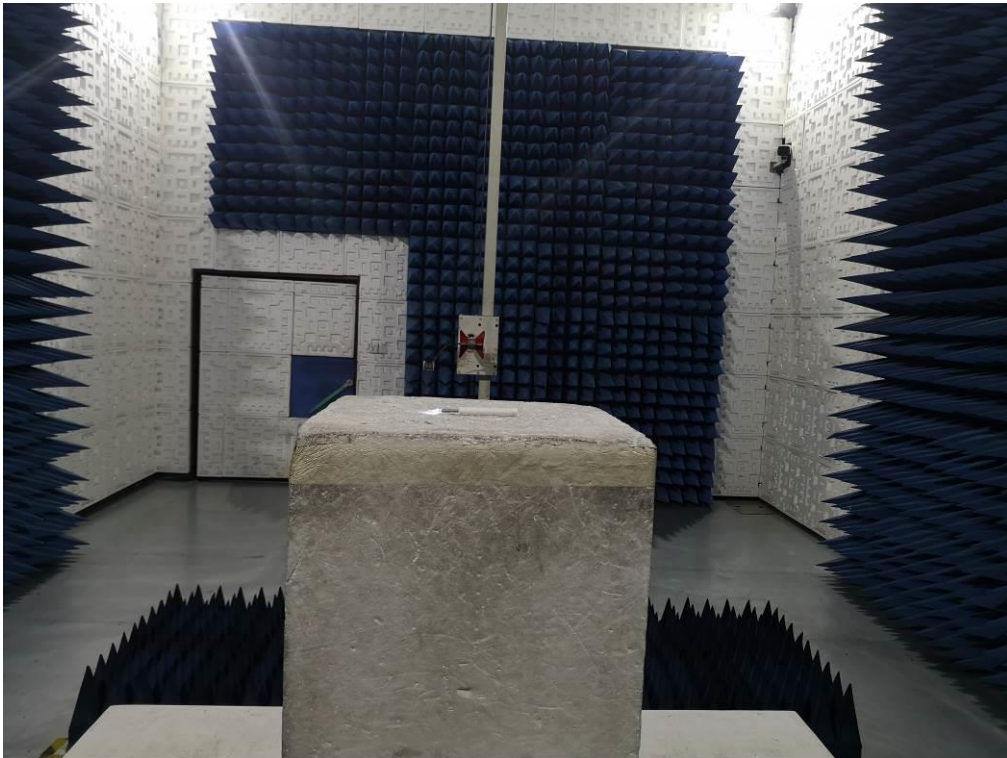
FCC RADIATED EMISSION TEST SETUP ABOVE 1GHZ
