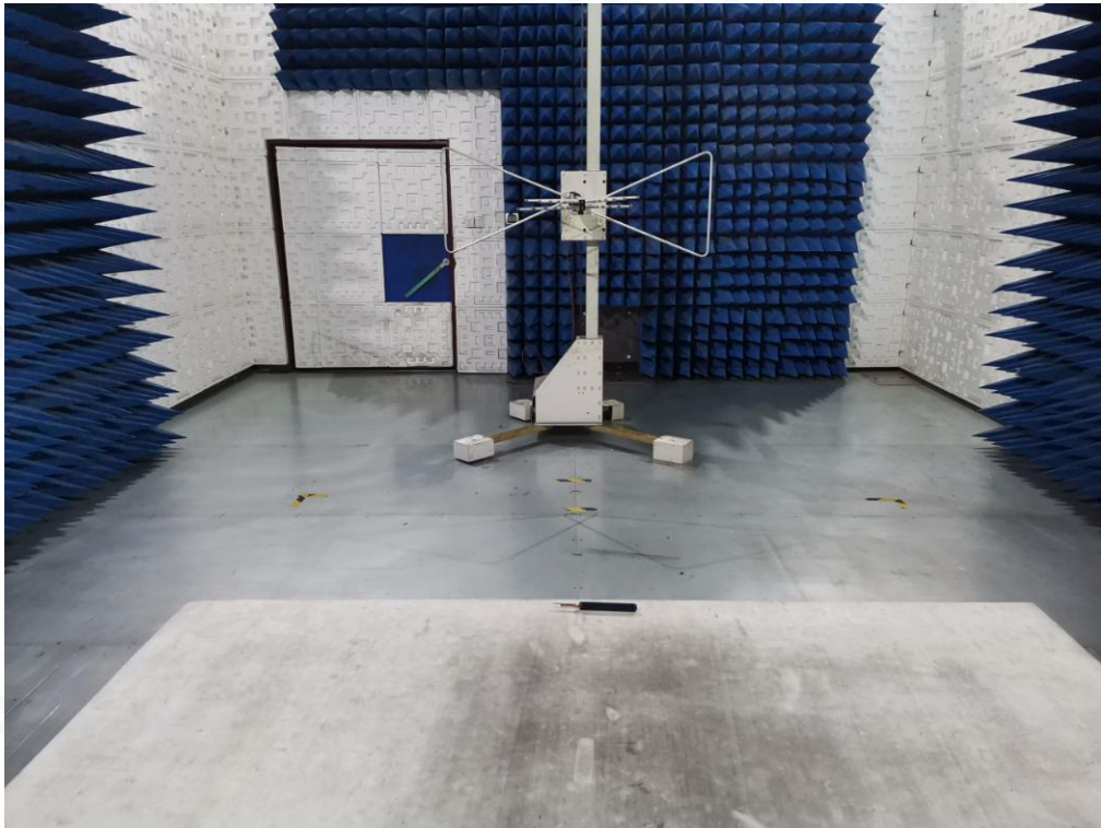
FCC RADIATED EMISSION TEST SETUP ABOVE 1GHZ
