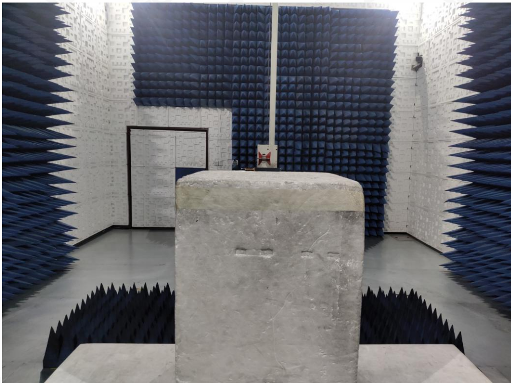
FCC RADIATED EMISSION TEST SETUP ABOVE 1GHZ
