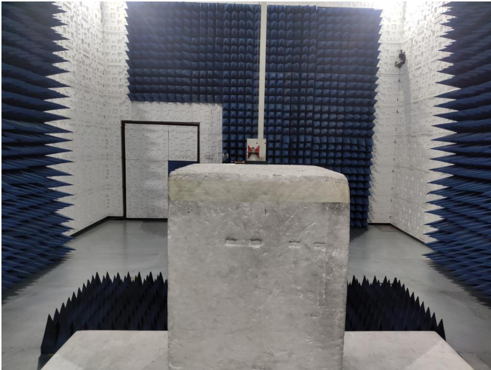
FCC RADIATED EMISSION TEST SETUP ABOVE 1GHZ
