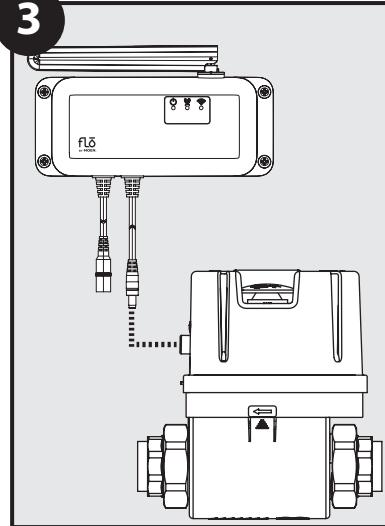
Using the long cable from the cellular antenna, plug the male connector into the female power connection on the Flo by Moen device. Rotate while inserting the plug until the plug is fully connected. Use of silicone lubricant is recommended on the plug body to simplify installation.
