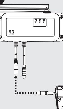
Plug the male connector from the Flo by Moen power adapter into the female socket on the short cable extending from the cellular antenna. Rotate while inserting the plug until the plug is fully connected.
