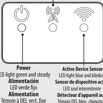
Once device is plugged in, wait for the green Power LED to remain solid, red Cellular Connection Status LED to remain solid and the blue Active Device Sensor LED to start blinking to indicate the cellular antenna is ready to pair with the Flo by Moen Smart Water Shutoff. **NOTE:** Upon Powering unit, device will be activated on cellular network. Power up sequence and cellular connection LEDs may take up to 5 minutes until solid.
