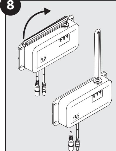
Position antenna so that it is pointing straight up to make a 90-degree angle with the housing.
