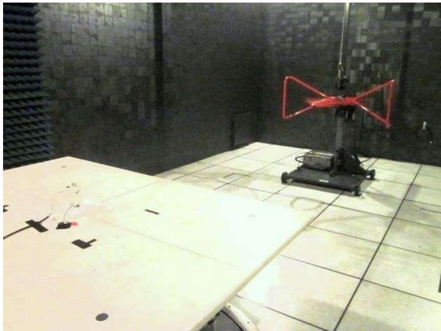
Radiated Emissions Test Setup 30 to 1000 MHz Shielded Room
