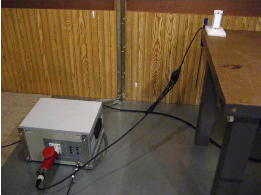
AC Mains Conducted Emissions Test Setup Picture
