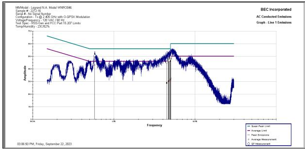
**Results:** All conducted emissions measured on the AC Power Port of the Legrand Model WNRCB46 Sample 2272-16 in Tx Mode Low Channel at 2.405 GHz are below the limit specified by FCC Part 15.207 and RSS-Gen 7.2 Limits by a margin of 2.83 dB.
