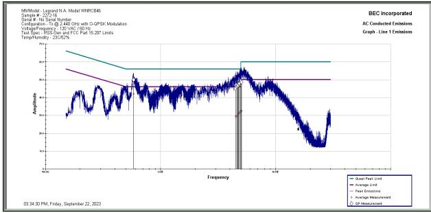
**Results:** All conducted emissions measured on the AC Power Port of the Legrand Model WNRCB46 Sample 2272-16 in Tx Mode Middle Channel at 2.440 GHz are below the limit specified by FCC Part 15.207 and RSS-Gen 7.2 Limits by a margin of 4.0 dB.
