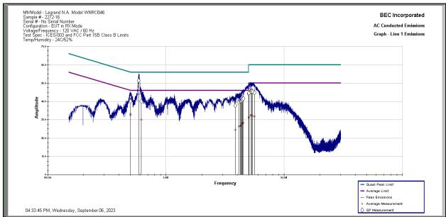
**Results:** All conducted emissions measured on the AC Power Port of the Legrand Model WNRCB46 Sample 2272-16 in Rx Mode are below the limit specified by FCC Part 15.207 and RSS-Gen 7.2 Limits by a margin of 1.93 dB.
