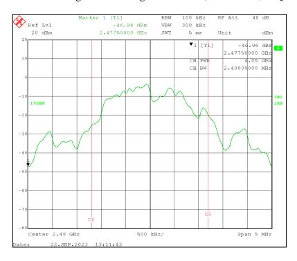
Legrand Model WNRCB46 Zigbee Radio Low Channel 11, 2.405 GHz, No modulation
