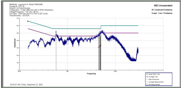
**Results:** All conducted emissions measured on the AC Power Port of the Legrand Model WNRCB46 Sample 2272-16 in Tx Mode High Channel at 2.480 GHz are below the limit specified by FCC Part 15.207 and RSS-Gen 7.2 Limits by a margin of 3.95 dB.
