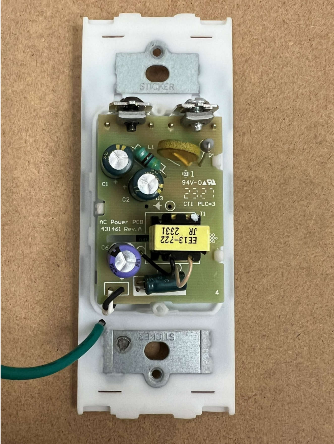
WNRCB46 AC Board Back Side
