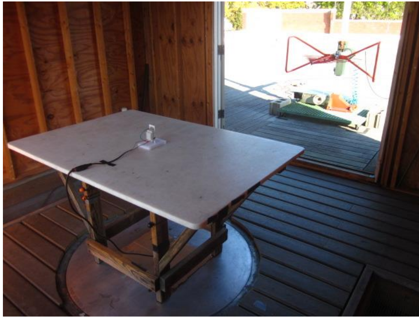
Radiated Emissions Test Setup 30 to 1000 MHz 3 Meter OATS
