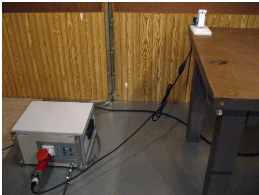
AC Mains Conducted Emissions Test Setup Picture
