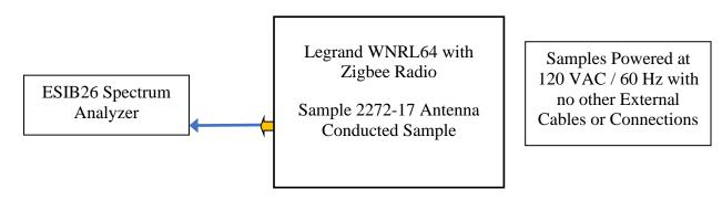
BEC-926, 1 Meter SMA Cable Connecting the SMA Connection from the Zigbee Radio Output to the Input of the Rohde and Schwarz ESIB26 Measurement Analyzer
