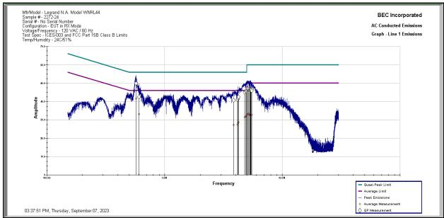
**Results:** All conducted emissions measured on the AC Power Port of the Legrand Model WNRL44 Sample 2272-24 in Rx Mode are below the limit specified by FCC Part 15.207 and RSS-Gen 7.2 Limits by a margin of 4.35 dB.
