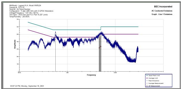
**Results:** All conducted emissions measured on the AC Power Port of the Legrand Model WNRL64 Sample 2272-18 in Tx Mode Low Channel at 2.405 GHz are below the limit specified by FCC Part 15.207 and RSS-Gen 7.2 Limits by a margin of 2.88 dB.
