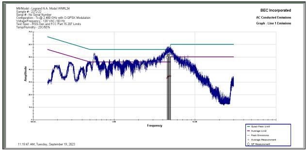
**Results:** All conducted emissions measured on the AC Power Port of the Legrand Model WNRL34 Sample 2272-22 in Tx Mode High Channel at 2.480 GHz are below the limit specified by FCC Part 15.207 and RSS-Gen 7.2 Limits by a margin of 4.58 dB.
