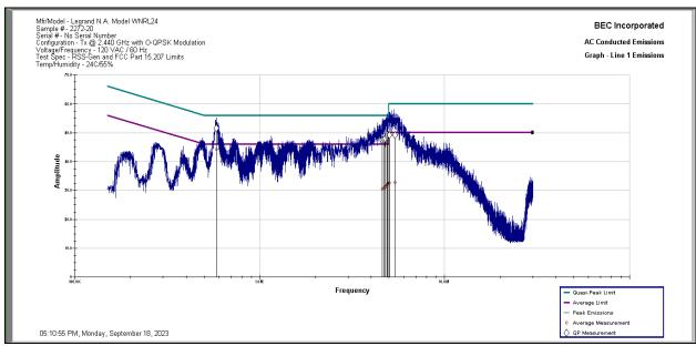
**Results:** All conducted emissions measured on the AC Power Port of the Legrand Model WNRL24 Sample 2272-20 in Tx Mode Middle Channel at 2.440 GHz are below the limit specified by FCC Part 15.207 and RSS-Gen 7.2 Limits by a margin of 1.76 dB.
