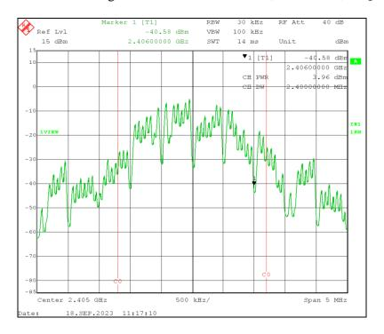
Legrand Model WNRL64 with Zigbee Radio Middle Channel 18, 2.440 GHz, O-QPSK Modulation
