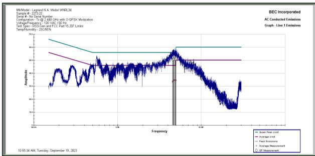
**Results:** All conducted emissions measured on the AC Power Port of the Legrand Model WNRL34 Sample 2272-22 in Tx Mode Middle Channel at 2.440 GHz are below the limit specified by FCC Part 15.207 and RSS-Gen 7.2 Limits by a margin of 4.61 dB.
