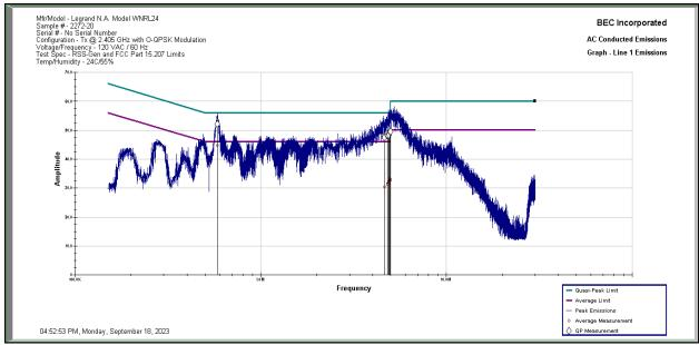
**Results:** All conducted emissions measured on the AC Power Port of the Legrand Model WNRL24 Sample 2272-20 in Tx Mode Low Channel at 2.405 GHz are below the limit specified by FCC Part 15.207 and RSS-Gen 7.2 Limits by a margin of 1.19 dB.
