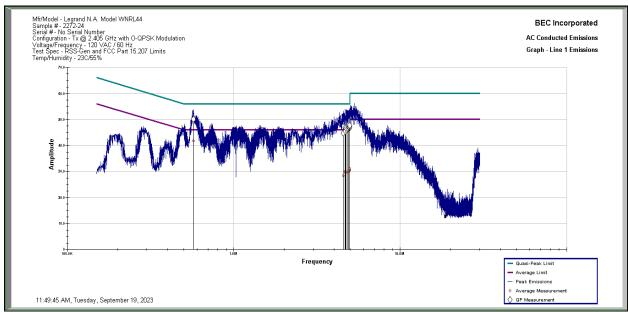
**Results:** All conducted emissions measured on the AC Power Port of the Legrand Model WNRL44 Sample 2272-24 in Tx Mode Low Channel at 2.405 GHz are below the limit specified by FCC Part 15.207 and RSS-Gen 7.2 Limits by a margin of 4.24 dB.
