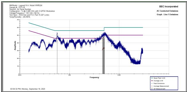
**Results:** All conducted emissions measured on the AC Power Port of the Legrand Model WNRL64 Sample 2272-18 in Tx Mode Middle Channel at 2.440 GHz are below the limit specified by FCC Part 15.207 and RSS-Gen 7.2 Limits by a margin of 3.63 dB.
