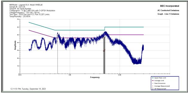
**Results:** All conducted emissions measured on the AC Power Port of the Legrand Model WNRL44 Sample 2272-24 in Tx Mode Middle Channel at 2.440 GHz are below the limit specified by FCC Part 15.207 and RSS-Gen 7.2 Limits by a margin of 4.50 dB.
