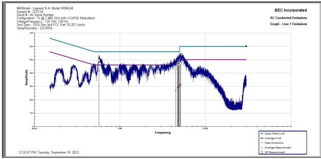
**Results:** All conducted emissions measured on the AC Power Port of the Legrand Model WNRL44 Sample 2272-24 in Tx Mode High Channel at 2.480 GHz are below the limit specified by FCC Part 15.207 and RSS-Gen 7.2 Limits by a margin of 4.41 dB.
