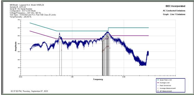
**Results:** All conducted emissions measured on the AC Power Port of the Legrand Model WNRL34 Sample 2272-22 in Rx Mode are below the limit specified by FCC Part 15.207 and RSS-Gen 7.2 Limits by a margin of 3.83 dB.
