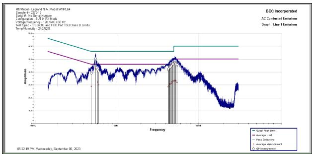
**Results:** All conducted emissions measured on the AC Power Port of the Legrand Model WNRL64 Sample 2272-18 in Rx Mode are below the limit specified by FCC Part 15.207 and RSS-Gen 7.2 Limits by a margin of 3.45 dB.
