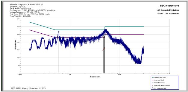
**Results:** All conducted emissions measured on the AC Power Port of the Legrand Model WNRL24 Sample 2272-20 in Tx Mode High Channel at 2.480 GHz are below the limit specified by FCC Part 15.207 and RSS-Gen 7.2 Limits by a margin of 1.91 dB.
