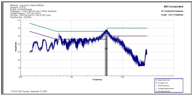
**Results:** All conducted emissions measured on the AC Power Port of the Legrand Model WNRL34 Sample 2272-22 in Tx Mode Low Channel at 2.405 GHz are below the limit specified by FCC Part 15.207 and RSS-Gen 7.2 Limits by a margin of 4.76 dB.
