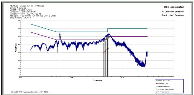
**Results:** All conducted emissions measured on the AC Power Port of the Legrand Model WNRL24 Sample 2272-20 in Rx Mode are below the limit specified by FCC Part 15.207 and RSS-Gen 7.2 Limits by a margin of 2.04 dB.
