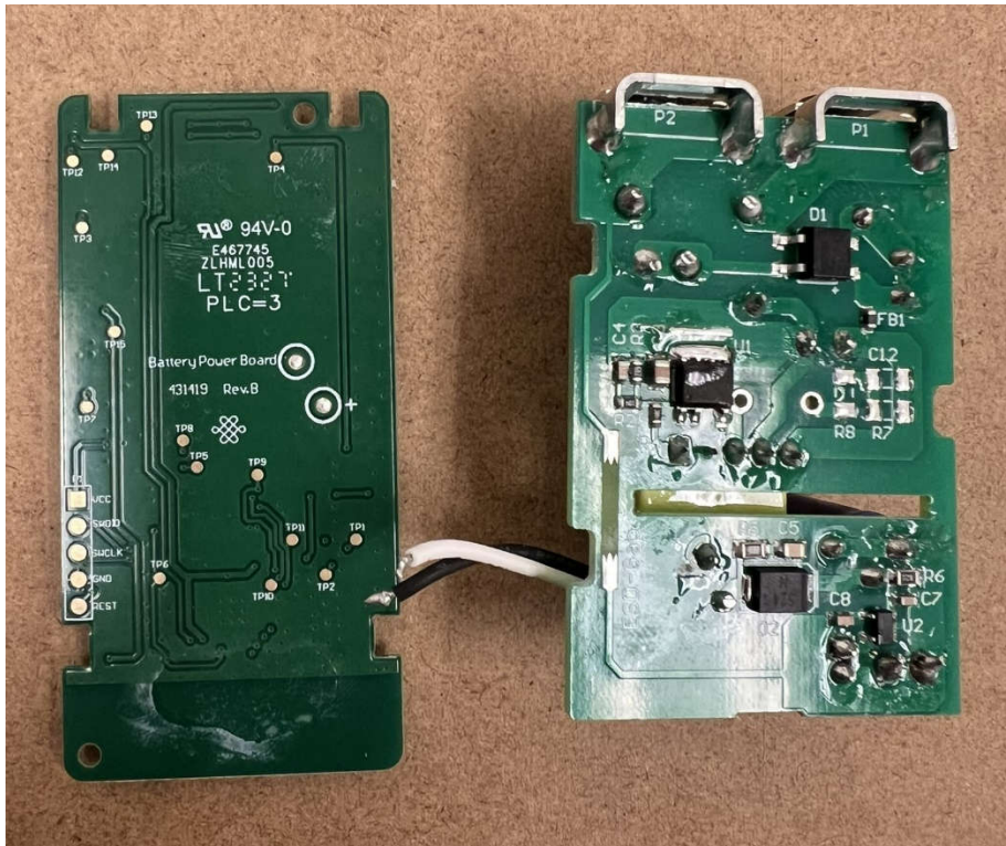
WZ3RL44 RF Board Back Side (Left) – AC Board Top Side (Right)
