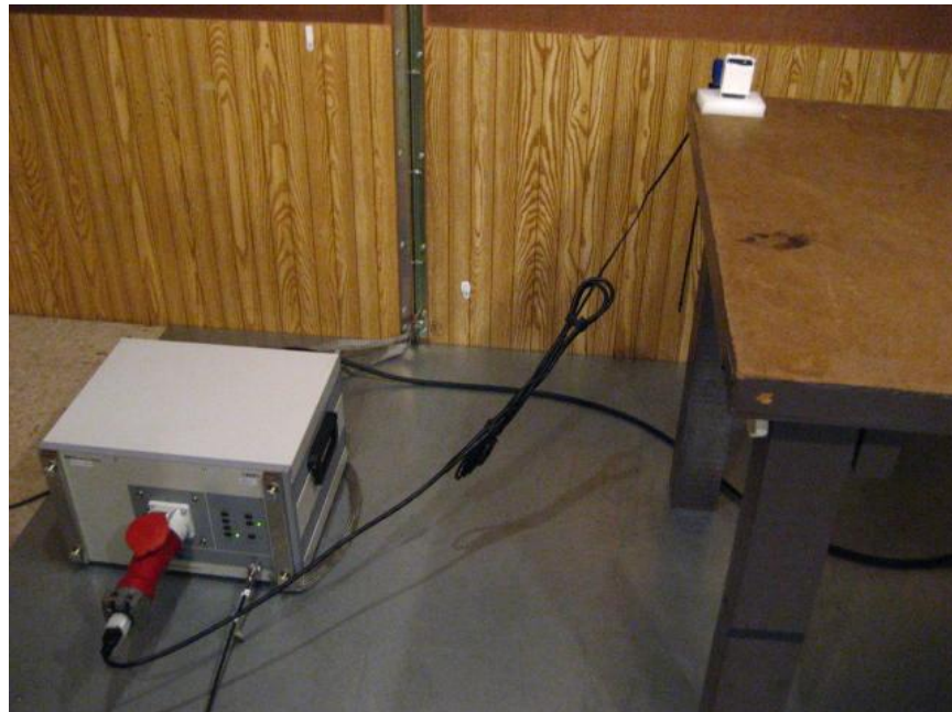
AC Mains Conducted Emissions Test Setup Picture
