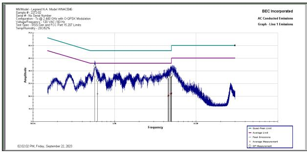
**Results:** All conducted emissions measured on the AC Power Port of the Legrand Model WNACB46 Sample 2272-02 in Tx Mode Middle Channel at 2.440 GHz are below the limit specified by FCC Part 15.207 and RSS-Gen 7.2 Limits by a margin of 10.61 dB.
