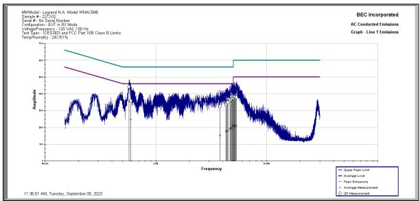
**Results:** All conducted emissions measured on the AC Power Port of the Legrand Model WNACB46 Sample 2272-02 in Rx Mode are below the limit specified by FCC Part 15.207 and RSS-Gen 7.2 Limits by a margin of 10.59 dB.
