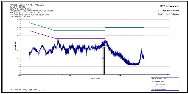
**Results:** All conducted emissions measured on the AC Power Port of the Legrand Model WNACB46 Sample 2272-02 in Tx Mode Low Channel at 2.405 GHz are below the limit specified by FCC Part 15.207 and RSS-Gen 7.2 Limits by a margin of 11.20 dB.
