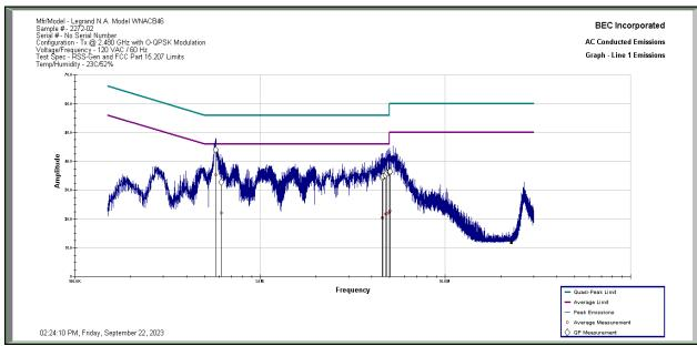
**Results:** All conducted emissions measured on the AC Power Port of the Legrand Model WNACB46 Sample 2272-02 in Tx Mode High Channel at 2.480 GHz are below the limit specified by FCC Part 15.207 and RSS-Gen 7.2 Limits by a margin of 10.65 dB.
