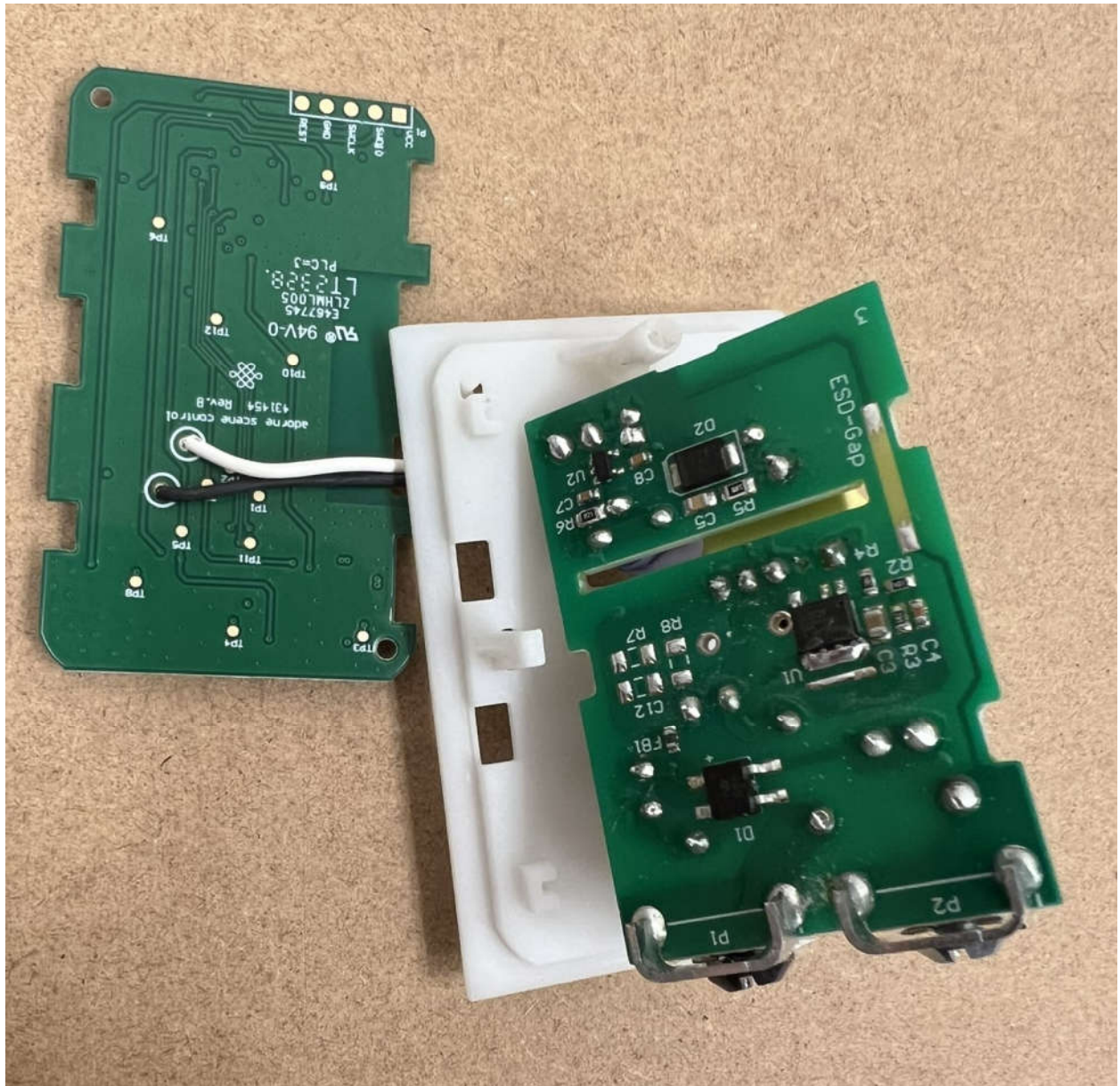
WZ3ACB46 RF Board Back Side (Left) – AC Board Top Side (Right)
