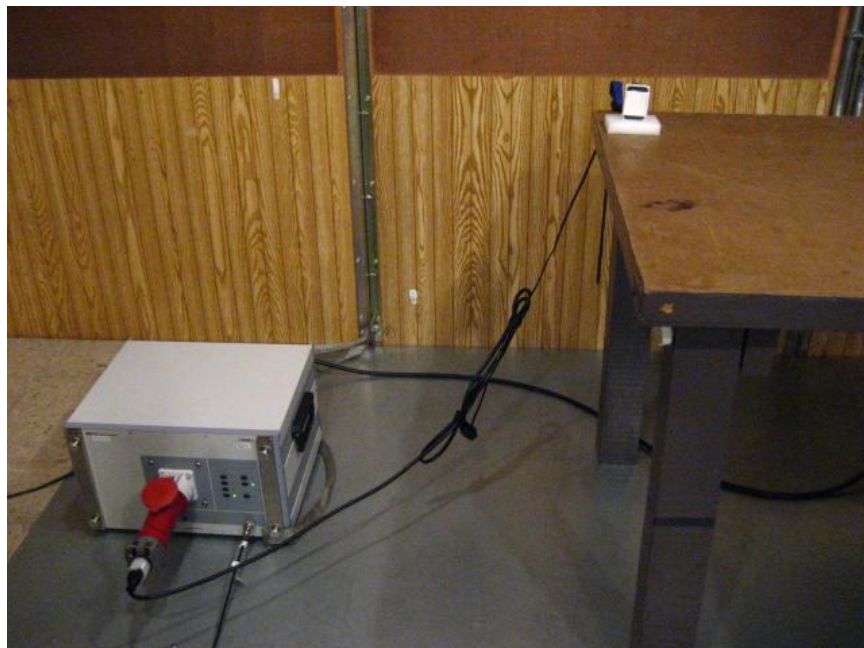
AC Mains Conducted Emissions Test Setup Picture
