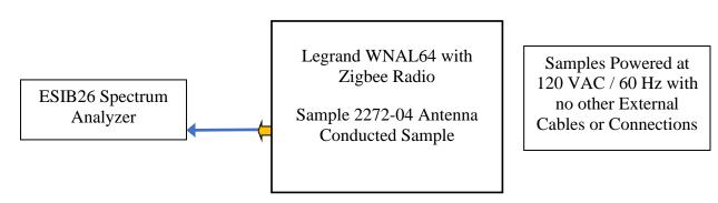
BEC-926, 1 Meter SMA Cable Connecting the SMA Connection from the Zigbee Radio Output to the Input of the Rohde and Schwarz ESIB26 Measurement Analyzer
