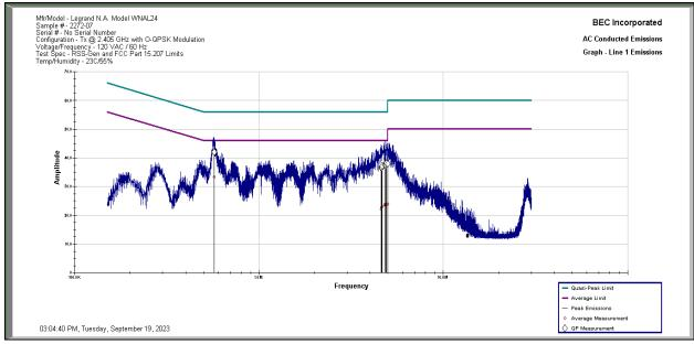
**Results:** All conducted emissions measured on the AC Power Port of the Legrand Model WNAL24 Sample 2272-07 in Tx Mode Low Channel at 2.405 GHz are below the limit specified by FCC Part 15.207 and RSS-Gen 7.2 Limits by a margin of 12.61 dB.
