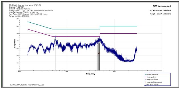
**Results:** All conducted emissions measured on the AC Power Port of the Legrand Model WNAL24 Sample 2272-07 in Tx Mode High Channel at 2.480 GHz are below the limit specified by FCC Part 15.207 and RSS-Gen 7.2 Limits by a margin of 12.2 dB.
