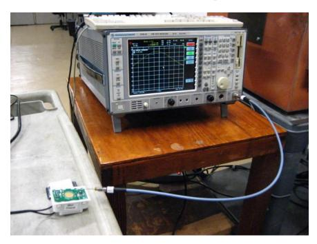
Antenna Conducted Test Setup Picture
