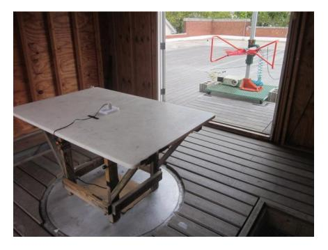
Radiated Emissions Test Setup 30 to 1000 MHz 3 Meter OATS
