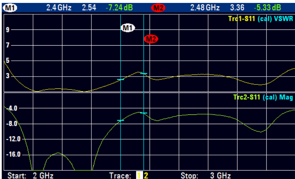
figure 3. WNAL23 antenna matching with the default matching Network
