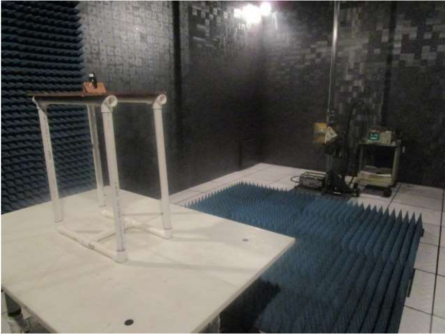
RADIATED EMISSIONS TEST SETUP 1 TO 18 GHZ
