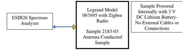
BEC-926, 1 Meter SMA Cable Connecting the SMA Connection from the Zigbee Radio Output to the Input of the Rohde and Schwarz ESIB26 Measurement Analyzer
