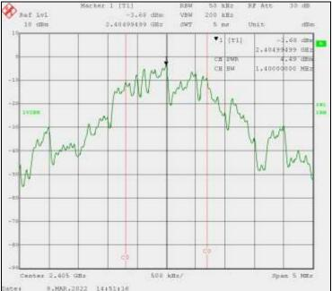
Legrand Model 067695 with Zigbee Radio Tx Middle Channel 18, 2440 MHz, O-QPSK Modulated
