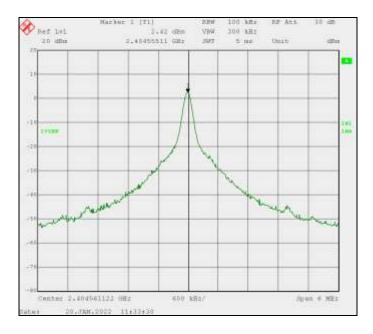
The peak level of 2.42 dBm is the maximum peak output of the Legrand Model 067695 with Zigbee Radio transmitting with modulation on Channel 11 at full power. The conducted spurious emissions from the antenna port must be 30 dB down from this peak. The resultant limit is therefore -27.6 dBm. This limit is displayed on the plots below.
