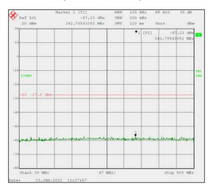
Legrand Model 067695 Zigbee Radio Transmitting Ch.11: 30 MHz – 500 MHz
