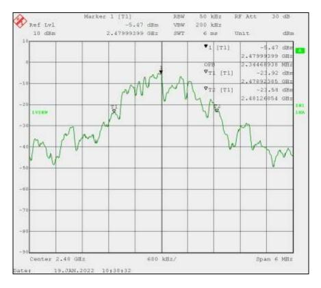
Legrand Model 067695 with Zigbee Radio 99% Occupied Bandwidth Summary Table
