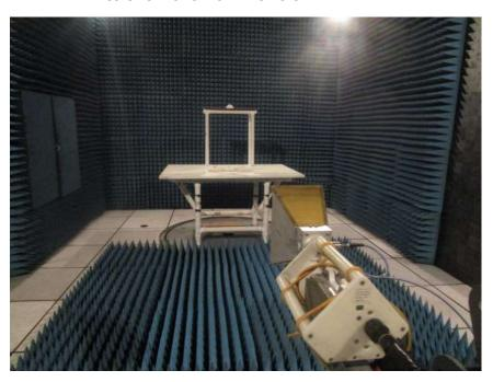
RADIATED EMISSIONS TEST SETUP 18 TO 25 GHZ
