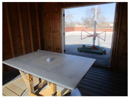
RADIATED EMISSIONS TEST SETUP 1 TO 18 GHZ
