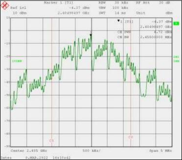
Legrand Model 064875 with Zigbee Radio Tx Middle Channel 18, 2440 MHz, O-QPSK Modulated
