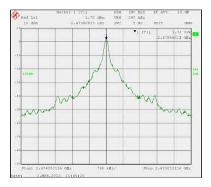
The peak level of 1.7 dBm is the maximum peak output of the Legrand Model 064875 with Zigbee Radio transmitting with no modulation on Channel 26 at full power. The conducted spurious emissions from the antenna port must be 30 dB down from this peak. The resultant limit is therefore -28.3 dBm. This limit is displayed on the plots below.
