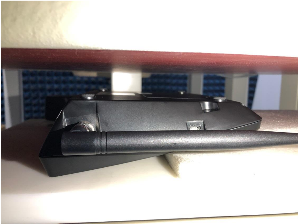
Back- Horizontal (the back of the device at a distance of 25mm from the flat phantom)
