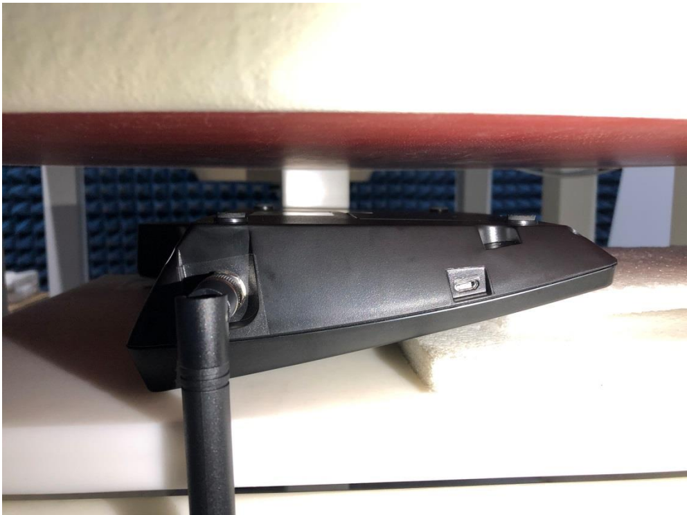
Back- Vertical (the back of the device at a distance of 25mm from the flat phantom)
