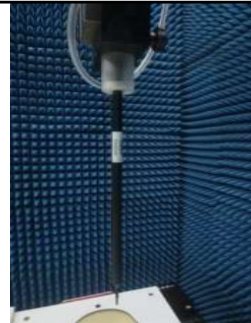
Fig.8.2 Photo of E-Field Probe
