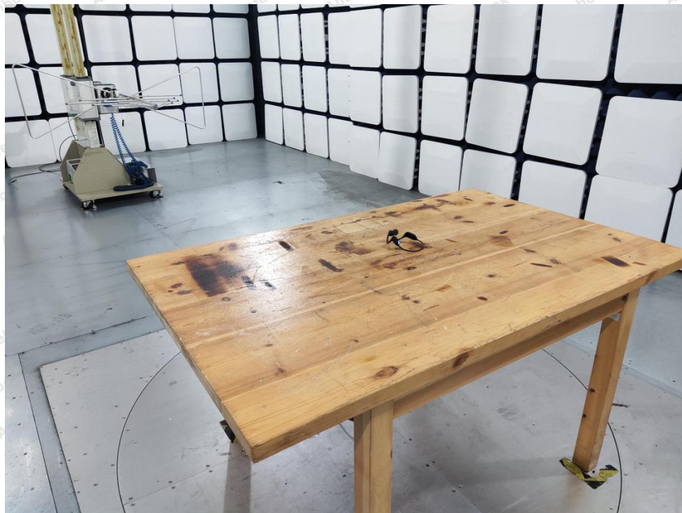
Photo of Radiation Emission Test
