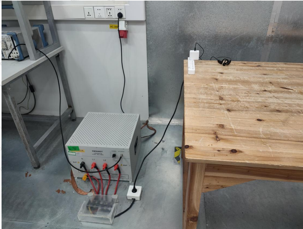
Photo of Conducted Emission Measurement
