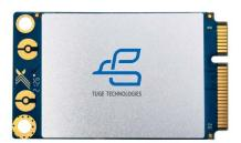
The TM22 Mini PCIe is an LTE module (data only) that supports the PCI Express Mini Card standard interface. TM22 module supports LTE CAT4 delivering 150Mbps downlink and 50Mbps uplink data rates. It also supports UMTS/HSPA technology, R99 WCDMA with a maximum downlink and uplink rate of 384Kbps, 3GPP R7 CAT14 HSDPA with 21Mbps and 3GPP R7 CAT7 HSUPA with 5.76Mbps.
