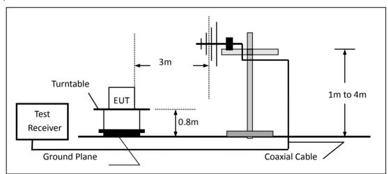
(c) For radiated emissions above 1000MHz
