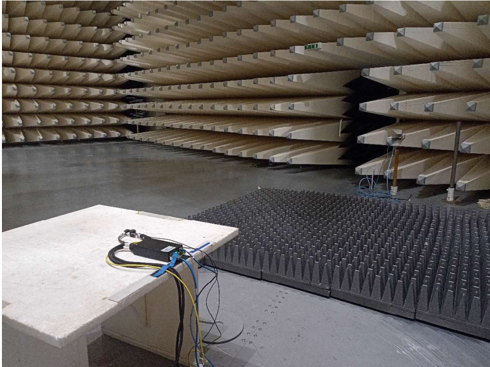
Photo 3: test setup of radiated emission >1GHz
