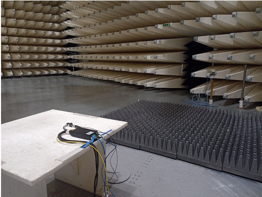
Photo 3: test setup of radiated emission >1GHz
