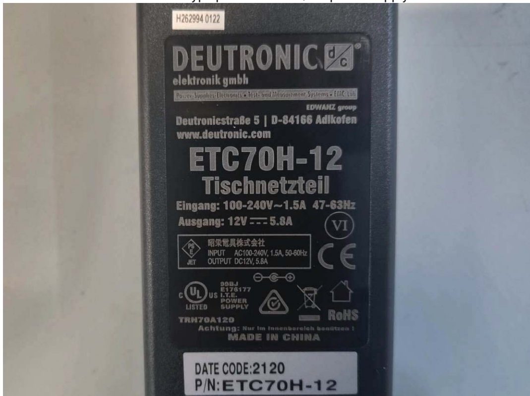
Photo 13: type plate of the AC/DC-power supply
