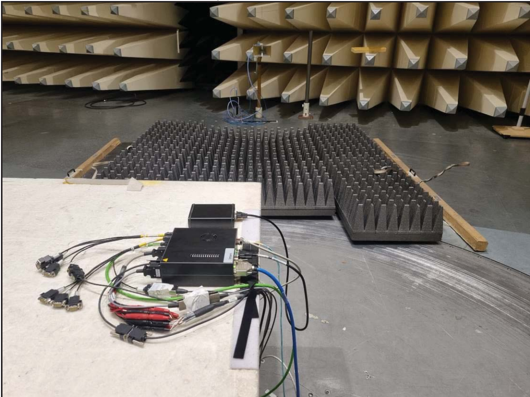
Photo 3: setup of radiated emission >1 GHz
