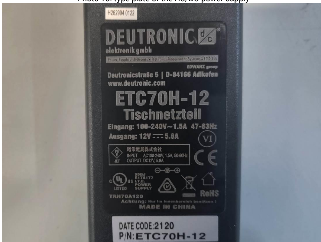
Photo 13: type plate of the AC/DC-power supply
