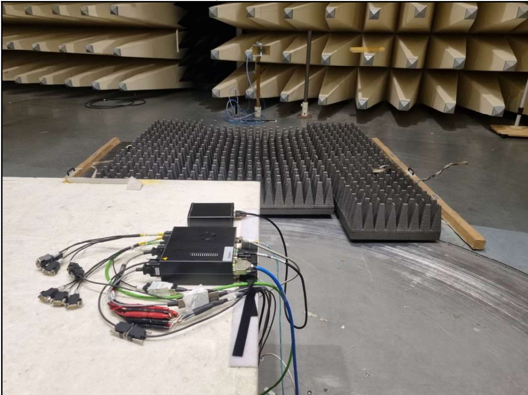
Photo 3: setup of radiated emission >1 GHz
