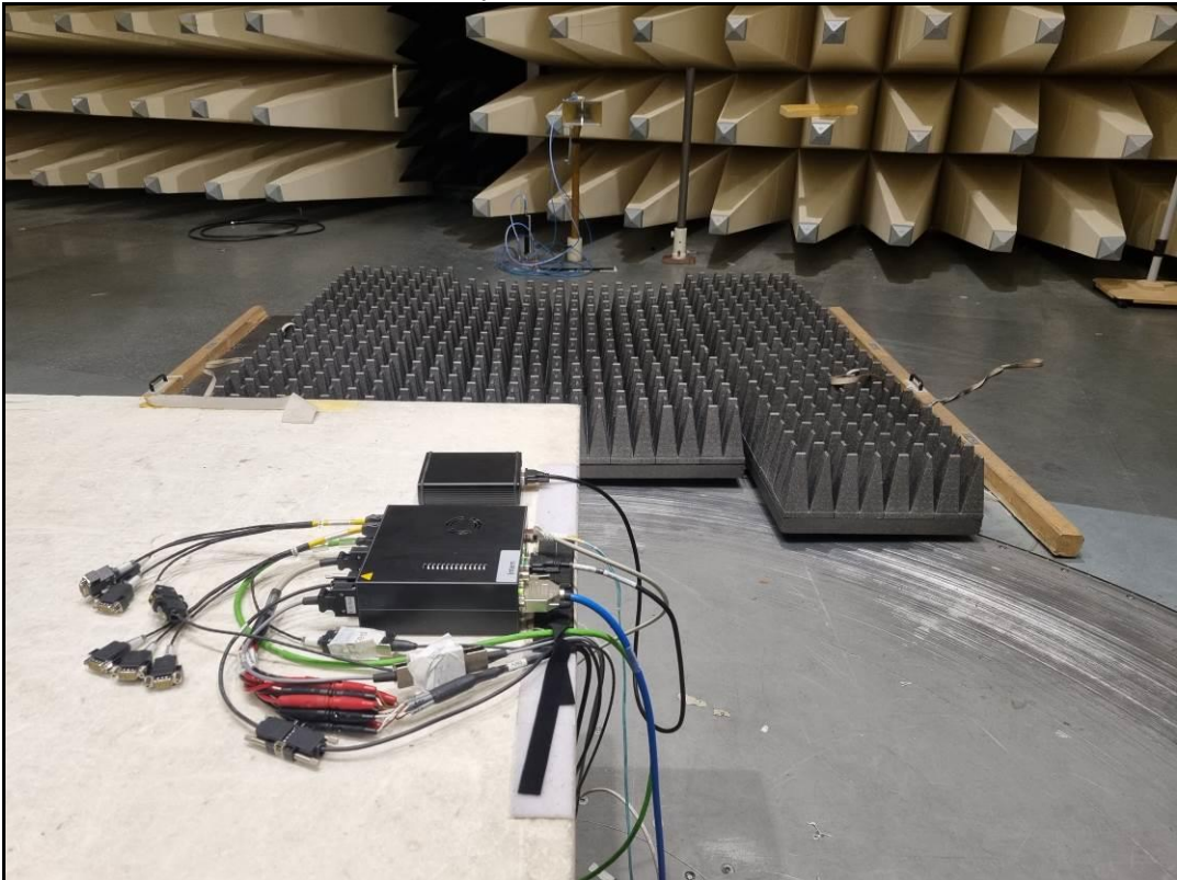
Photo 3: setup of radiated emission >1 GHz
