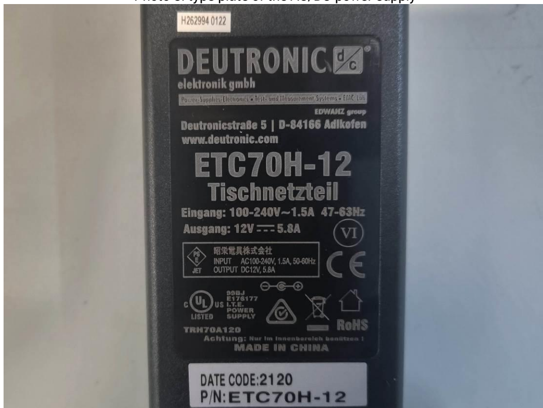
Photo 8: type plate of the AC/DC-power supply
