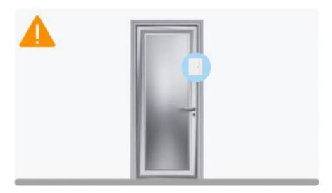
Please install carefully on metal doors and windows, as the device's performance will be significantly affected and may also cause wireless signal interference leading to disconnection.
