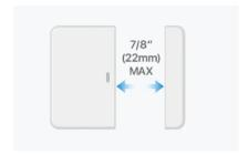
The sensor and magnet must be aligned, and the distance between them should be as small as possible, with a maximum distance not exceeding 3/4" (20 mm). Metal doors and windows have a significant impact on the device, and when installed on metal doors and windows, the distance between the sensor and magnet needs to be further reduced.
