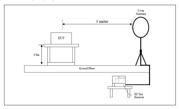
Radiated Emission Test-Up Frequency 30MHz~1GHz/Above 1GHz
