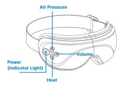
() : Press and hold to turn on/off the device. Mode 1 (Air Pressure plus Heat) will be activated by default. The indicator light will be solid white.
