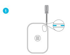
Insert flat screwdriver into special hole and lift.
