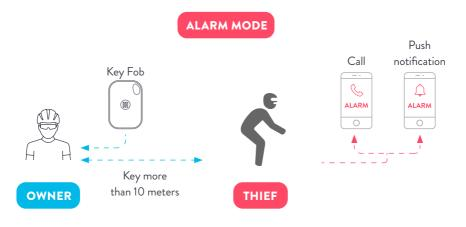
When in alarm mode MONIMOTO9U first calls the owner's number. It will call ONCE and after that you will start receiving push notifications to the MONIMOTO9U app. You will see a GPS location if precise location data is received or an approximate location from LTE network triangulation using Cell ID if GPS is not available.
