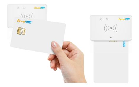
3. When the blue light flashes, it means the card and the reader is performing data communication
