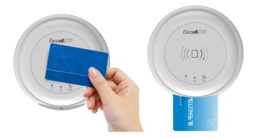
3. When the light flashes, it means the card and the reader is performing data communication (blue light for contact, green light for contactless).
