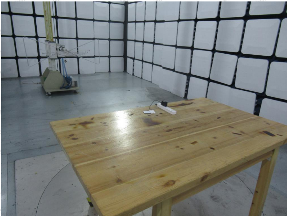
Photo of Radiation Emission Test
