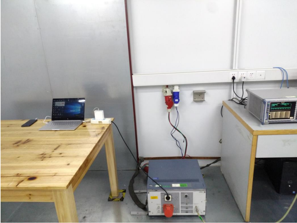
FCC RADIATED EMISSION TEST SETUP
